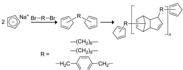
**Scheme 34.** Copolymerization of Biscyclopentadienes with *p*-Benzoquinone.<sup>142</sup>
