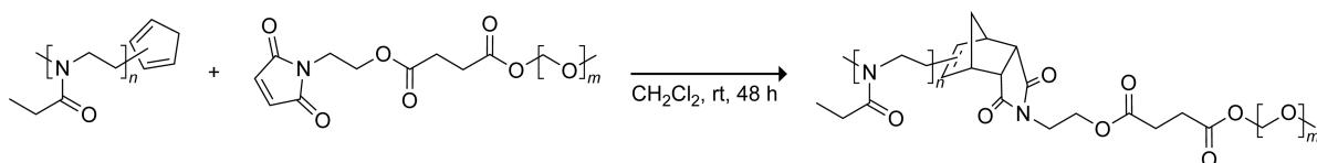
**Scheme 37.** Diblock Copolymer Synthesis from the Diels–Alder Reaction of a Maleimide-Functionalized Polymer with a Cyclopentadiene-Functionalized Polymer Generated from the Reaction of a Tetrazine and a Norbornadiene<sup>148</sup>
