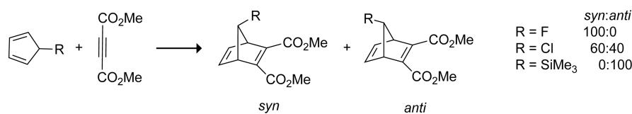
trimethylsilylcyclopentadiene<sup>43</sup> provides exclusively the *anti* cycloadduct, and 5-chlorocyclopentadiene<sup>44</sup> provides a mixture of the *syn* and *anti* cyclic adducts (Scheme 8).
